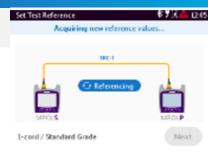
Connect the MPOLP to the MPOLS using an **UNPINNED-to- UNPINNED** MTP Pro connectorized test reference cord (TRC-1) as shown below.
