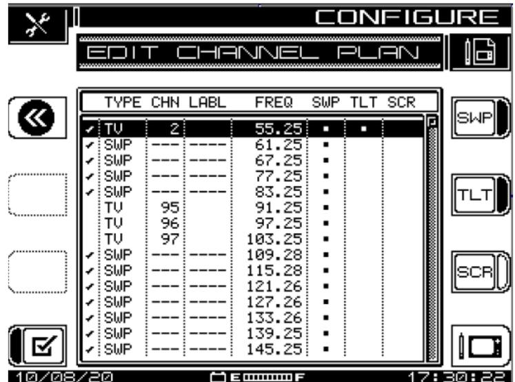
**Step 15A:** This step is to change TV Carrier to QAM digital Stream.
