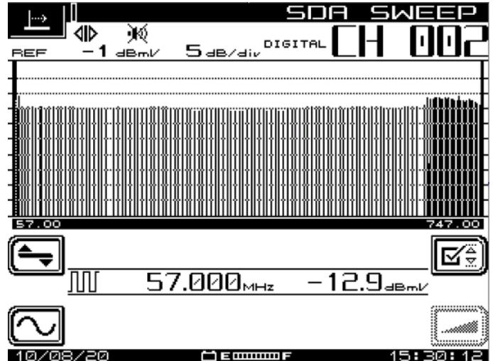
**Step 25:** The level of the Sweep insertion is accurate. **Should be stable**
