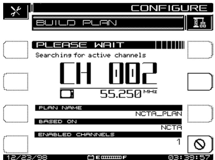
**Step 8:** The Channel plan has been built.
