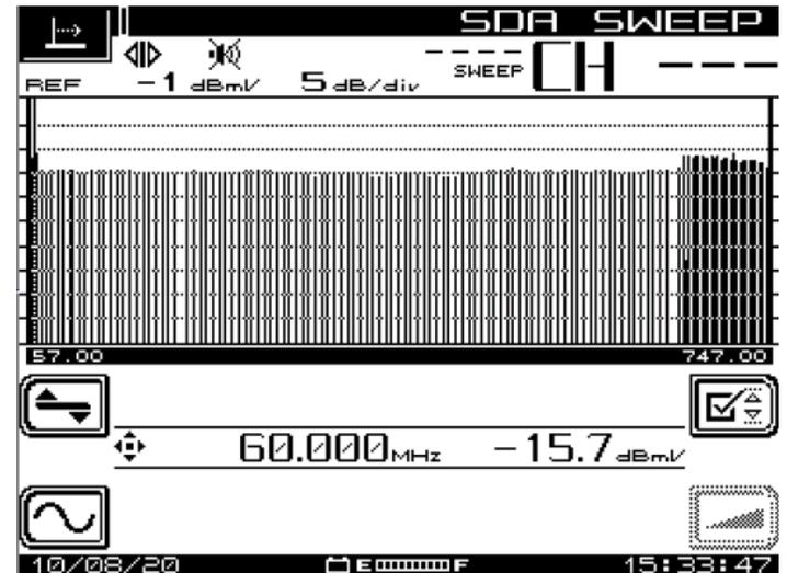
**Step 26:** Note the level of OFDM carriers in your plan. They may read inaccurate in the sweep mode due to the algorithm for level stability. **Should be stable**
