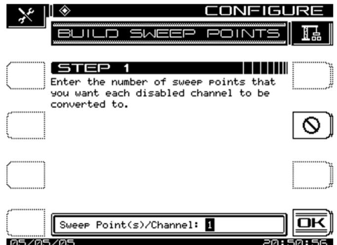
**Step 11:** Turns no active carriers into sweep injections.
