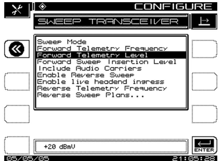
**Step 21:** Set Forward sweep insertion to the lowest setting of 20.
