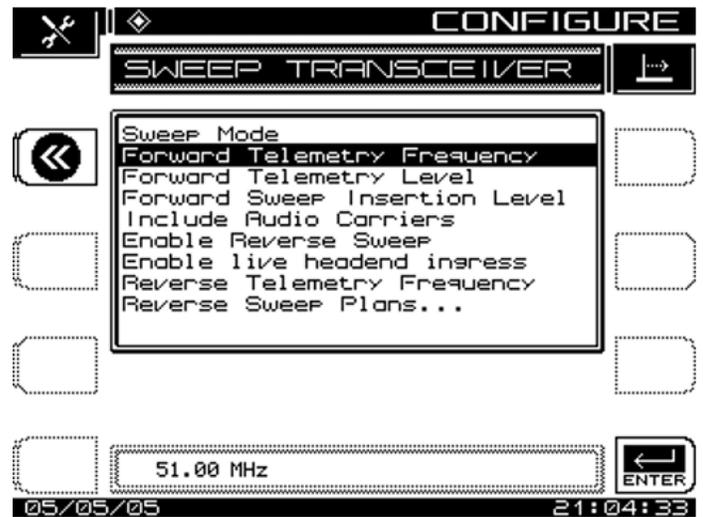
**Step 20:** Set Forward telemetry to the lowest setting of 20.
