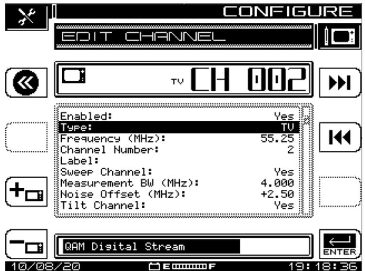
**Step 15B:** Edit QAM carrier and OFDM in 6 MHz increments
