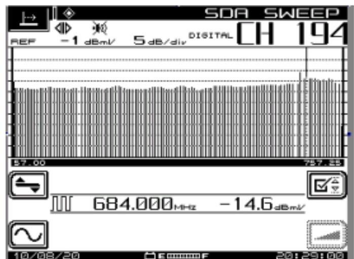
**Step 27: Forward Absolute and Referenced Sweep Max Min on Referenced sweep < .8 typical**
