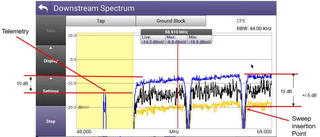
Note: If Sweep trace is too noisy after reference > 1 dB P/V then raise the sweep insertion level according.
